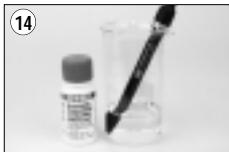
Older sensors can be regenerated by placing them for 12 hours into a KCL solution (immerse the tip of the sensor about 2 cm) **(14)**. Then rinse the sensor with distilled water and calibrate again. Employing this process, it may also be possible to regenerate sensors which had dried out due to an oversight.
