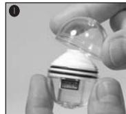
2. Take an ampoule of special CO<sub>2</sub> indicator and ensure that there is no indicator in the neck of the ampoule! For this purpose, shake the indicator down to the bottom of the ampoule (in the same manner as a thermometer is shaken before taking someone's temperature). Open ampoule by twisting off the sealing tab.
